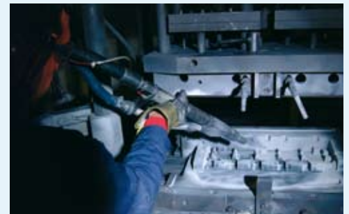
Alumina based die coating removal at 300°C
