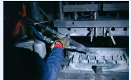
Alumina based die coating removal at 300°C
